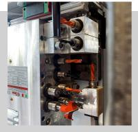
5 drills, 32mm system, individual activation (4 vertical alignment, 2 horizontal alignment)
