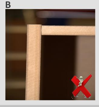
B.— Bad joints produced by differences in the length and squaring of the piece (machines without Electronic squaring probe)
