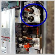
2 drill units in horizontal direction (X) to make edge holes, at right and left side.
