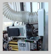
High frequency motor, 18000rpm, 3 hp, to make routing, milling, cuts, slots, decorative design, corners retails, Gola arcs, and more. It replace the saw unit to make the groove, because is faster, only one pass to finish the width of the groove using the right tool
