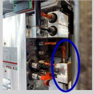
1 drill unit to make holes by the down edge of the piece. Also this unit is useful for the machine to press the piece when the clamp needs to move position. This unit is required to make the hole to fit the brake or soft spring for doors or drawers
