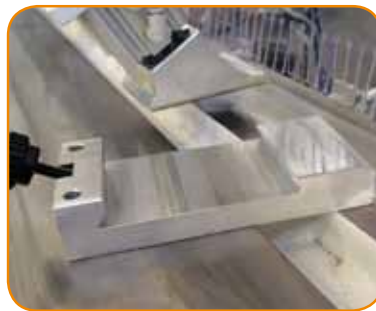
Clamp pad extension for pressing pieces minimum width 40 mm.
