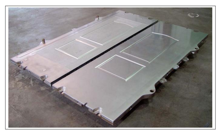
• Core and cavity set of doorskin mold
